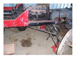
Ts) and had to make up the linkage as that was missing. The body was in good condition. Stripped all the paint and replaced the rear seat support and painted twice (Valmay can pick a paint run at 100 metres). The mother-in-law seat is a tub chair cut down with timber inserts fitted.
