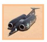
The car is powered by two Rolls-Royce Spey 202 jet engines which generate 222 kN of thrust.
